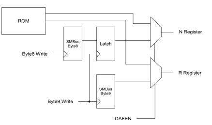
Figure 1. Dial-a-Frequency Register Loading
