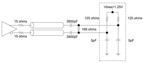
Figure 2. Test Load Configuration
