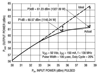
Figure 7. Pulsed Output Power versus Input Power
