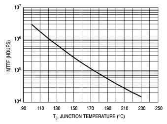
This above graph displays calculated MTTF in hours when the device is operated at V<sub>DD</sub> = 50 Vdc, P<sub>out</sub> = 1000 W Peak, Pulse Width = 100  $\mu sec$ , Duty Cycle = 20%, and  $\eta_D$  = 71%.
