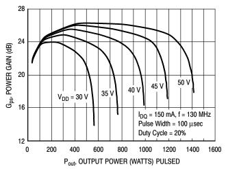
Figure 9. Pulsed Power Gain versus
