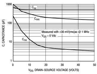
Figure 4. Capacitance versus Drain-Source Voltage
