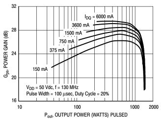
Figure 8. Pulsed Power Gain versus
