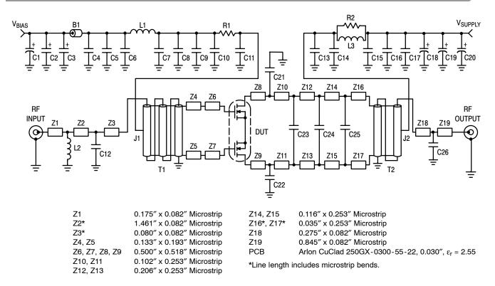
Figure 2. MRF6VP11KHR6 Test Circuit Schematic
