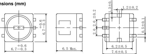
\* Dimension does not include solder used on coil. \* Pin pitch shall be measured at the root of terminal.
