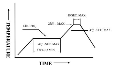
**DIP soldering (Wave Soldering)**
