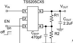
Adjustable Version:  $V_{OUT} = 1.24 (R1+R2)/R1$  (Adjustable output range up to 8V)
