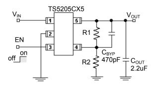
Adjustable Version: V<sub>OUT</sub> = 1.24 (R1+R2)/R1 (Adjustable output range up to 8V)
