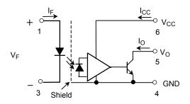
Note. A 0.1µF bypass capacitor must be connected between pins 4 and 6.
