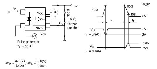
$C_{\text{L}}$  is approximately 15pF which includes probe and stray wiring capacitance.
