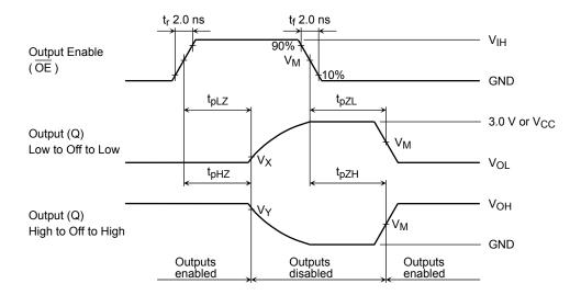
Figure 3  $t_{pLZ}, t_{pHZ}, t_{pZL}, t_{pZH}$
