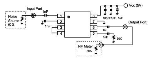
Figure 3 Measurement circuit
