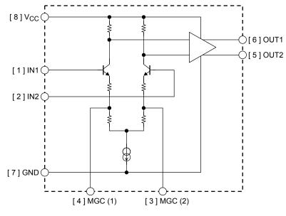
Figure 5 Equivalent circuit
