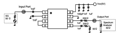
Figure 1 Measurement circuit (MGC:Short)
