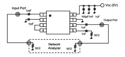
Figure 4 Measurement circuit
