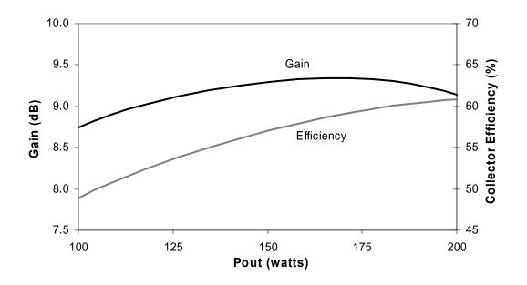
RF Power Transfer Curve 1090 MHz, Gain & Efficiency vs. Output Power
