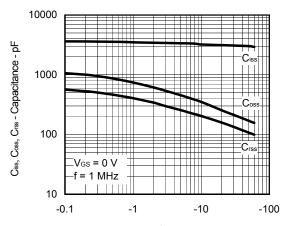
V<sub>DS</sub> - Drain to Source Voltage - V
