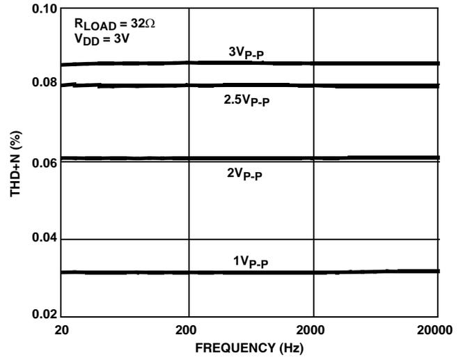
FIGURE 11. THD+N vs SIGNAL LEVELS vs FREQUENCY
