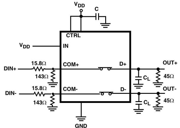
$|t_{ro} - t_{ri}|$  Delay Due to Switch for Rising Input and Rising Output Signals.
