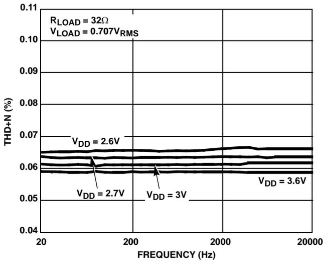
FIGURE 10. THD+N vs SUPPLY VOLTAGE vs FREQUENCY
