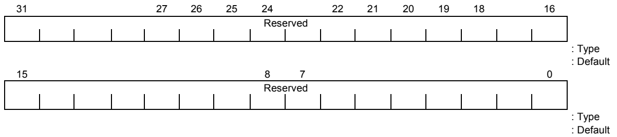
Power Management Function Register (PM_Cap) 0x40
