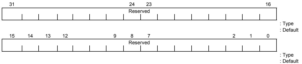
Power Management Control, Status Register (PM_CSR) 0x44
