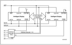
Multiple displays can be cascaded using the  $\overline{\text{CLKSEL}}$  and CLK I/O pins (Figure "Cascading Multiple Display"). The display designated as the MasterClock source should have its  $\overline{\text{CLKSEL}}$  pin tied high and the slaves should have their  $\overline{\text{CLKSEL}}$  pins tied low. All CLK I/O pins should be tied together. One display CLK I/O can drive 15 slave CLK I/Os. Use  $\overline{\text{RST}}$  to synchronize all display counters.
