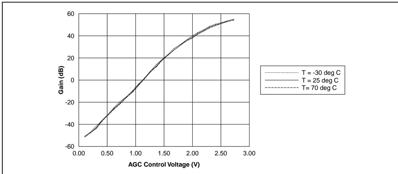
Figure 4 - FM Gain v AGC Voltage
