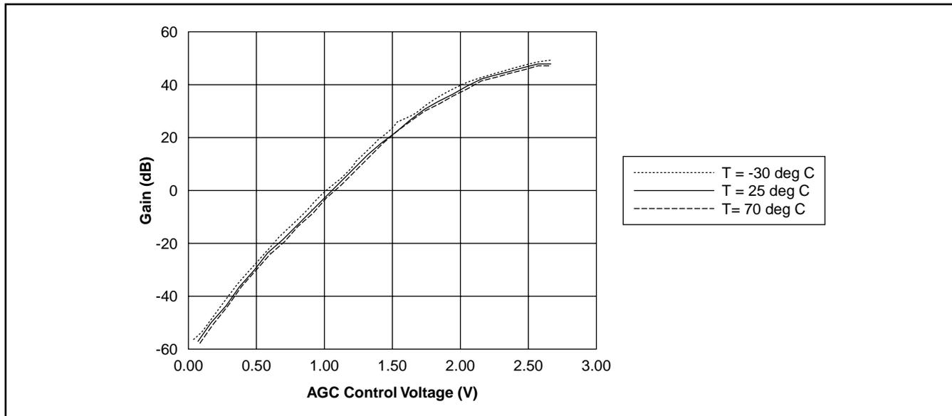
Figure 3 - CDMA Gain v AGC Voltage
