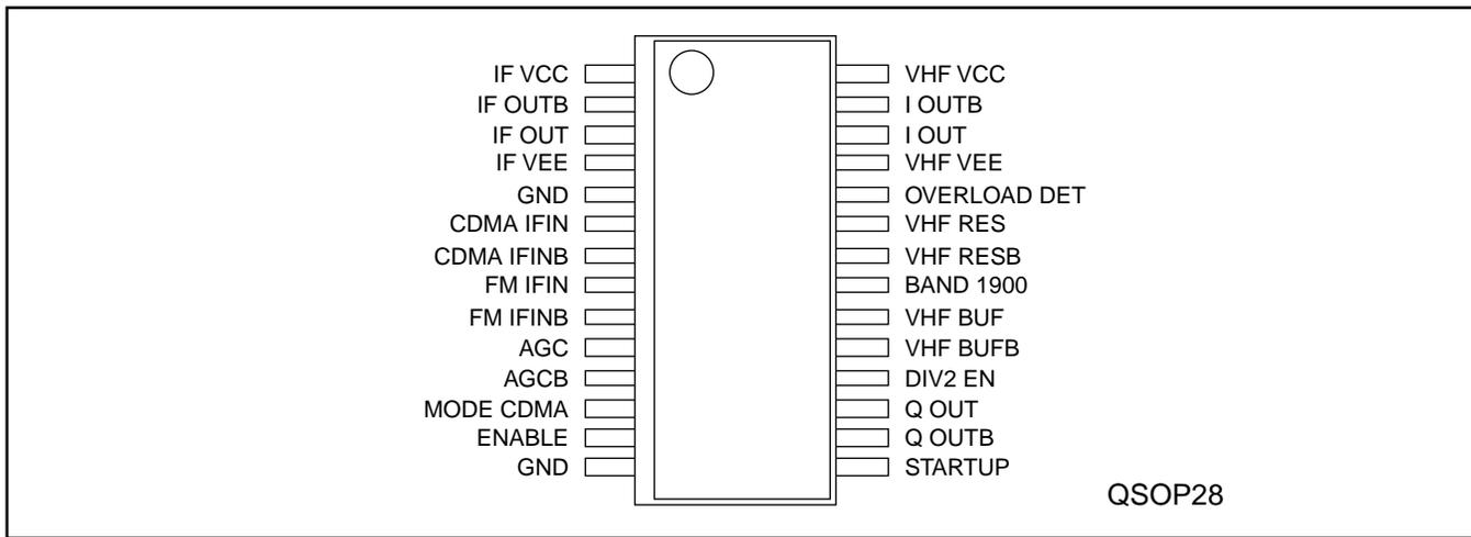
**Figure 2 - Pin Connections**
