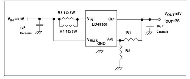
Figure 3. Single supply voltage solution
