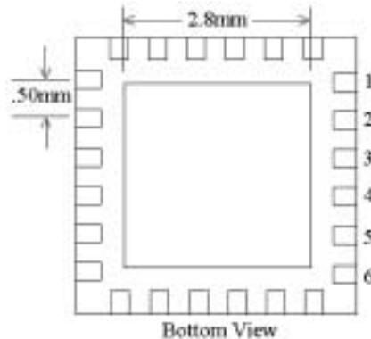
This package conforms to the LPCC<sup>™</sup> 4 x 4 mm 24 lead body dimensions. See ASAT LPCC Marketing Outline Dwg. # DGMJ00004 Latest Rev. at <http://www.asat.com> for additional dimensional information.
