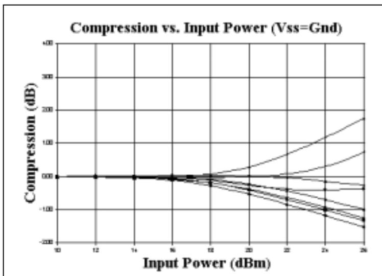
The P1dB curve shows all states with a P1dB compression at approximately 23dB input power. The conditions for this curve are  $V_{dd} = +5.0v$  and  $V_{ss} = 0v$ . For higher P1dB compression values, supply  $V_{ss}$  with a negative voltage as shown in the next curve.
