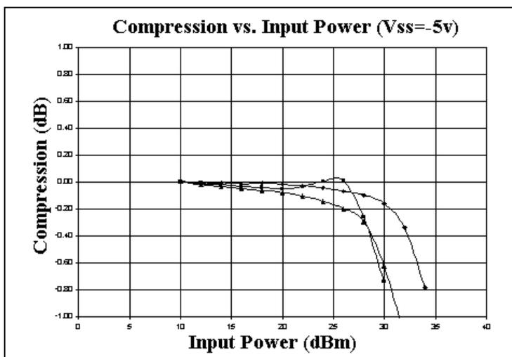
The P1dB curve shows all states with a P1dB compression at approximately 31dB input power. The conditions for this curve are  $V_{dd} = +5.0v$  and  $V_{ss} = -5.0v$ .
