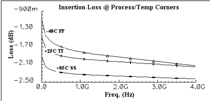
This Insertion Loss curve represents the Min/Max conditions for the "0" pass state versus all processing and temperature conditions. The Min case is at -40C with the "Fast" processing conditions. The Max case is at +85C with the "Slow" processing conditions. All other combinations fall within that band. The typical 25C case is labeled +25C TT.
