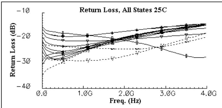
This Return Loss set of curves represents the combination of all Return Loss cases for all attenuation settings. All cases are better than -14dB Return Loss at 4GHz.
