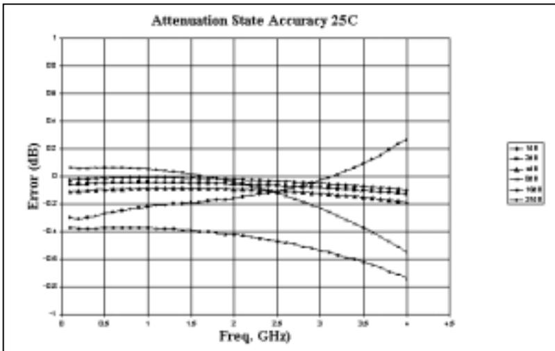
The Attenuation Accuracy curve with vertical axis of +/- 1dB shows all states better than +/- 0.5dB to 2GHz and better than +/- 0.8dB to 4GHz.
