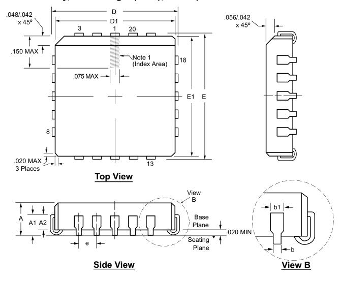
**Note 1:**A Pin 1 identifier must be located in the index area indicated. The Pin 1 identifier may be either a mold, or an embedded metal or marked feature.
