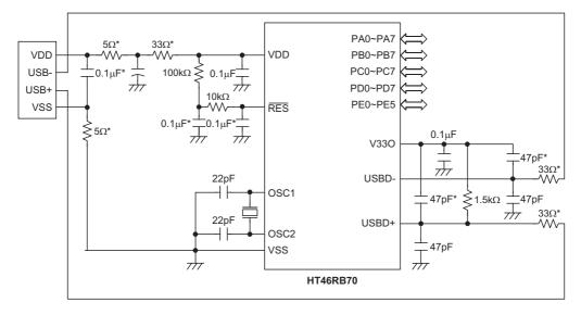
Note: The resistance and capacitance for reset circuit should be designed in such a way as to ensure that the VDD is stable and remains within a valid operating voltage range before bringing RES to high.
