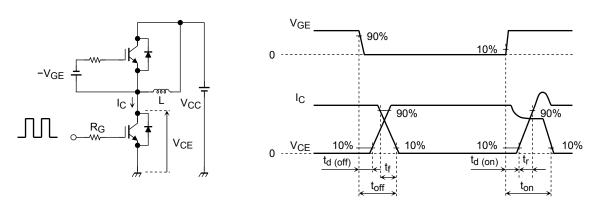
Note 2: Switching loss measurement waveforms
