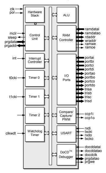
**Timer 0** – Main system's timer and prescaler. This timer operates in two modes: 8-bit timer or 8-bit counter. In the "timer mode", timer registers are incremented every 4 CLK periods. When the prescaler is assigned into the TIMER prescale ration can be divided by 2, 4 .. 256. In the "counter mode" the timer register is incremented every falling or rising edge of T0CKI pin, dependent on T0SE bit in OPTION register.
