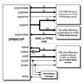
The described above implementation should be treated as an example. All Program Memory spaces are fully configurable. For timing-critical applications whole program code can be implemented as on-chip ROM and (or) RAM and
