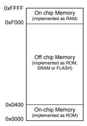
The figure below shows a typical Program Memories connections in system with DP8051XP Microcontroller core.
