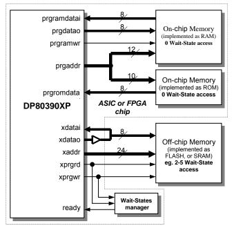
The described above implementation should be treated as an example. All Program Memory spaces are fully configurable. For timing-critical applications whole program code can be implemented as on-chip ROM and (or) RAM and executed without Wait-States, but for some
