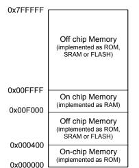
The figure below shows a typical Program Memories connections in system with DP80390XP Microcontroller core.
