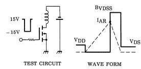
$R_G = 25\Omega$  $V_{DD} = -50V$ , L=1.44mH
