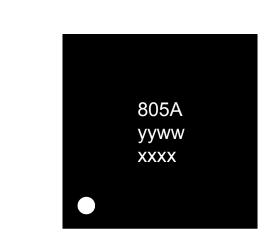
Marking for the 3x3mm MLPD-10 Lead Package: nnnn = Part Number (Example: 805A) yyww = Datecode (Example: 0652) xxxx = Semtech Lot No. (Example: E901)
