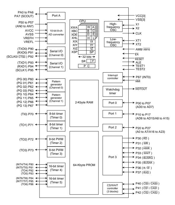
Figure 1.3 TMP93PS40 Block Diagram
