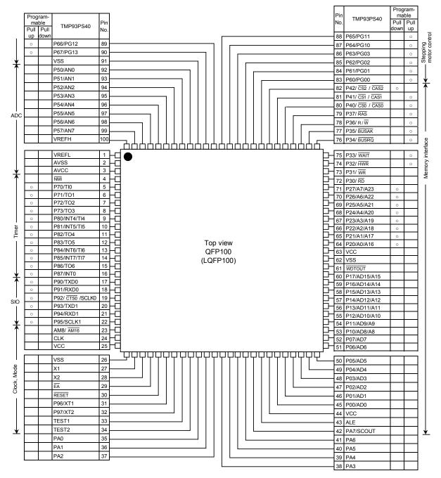
Figure 2.1.1 Pin Assignment (100-Pin QFP, 100-Pin LQFP)
