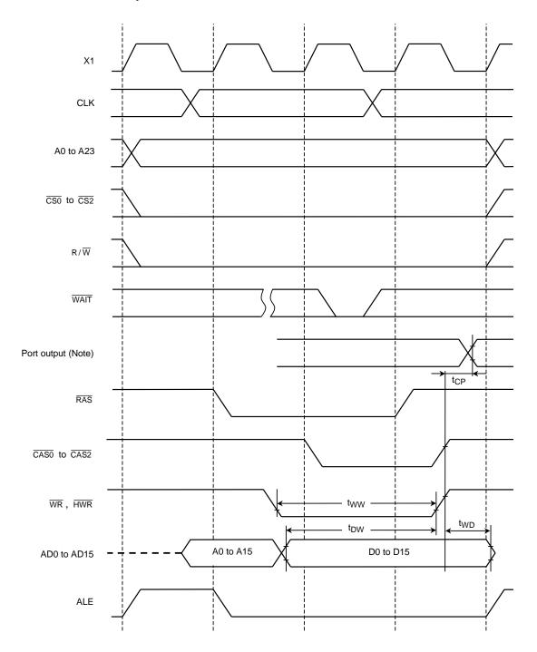
Note: Since the CPU accesses the internal area to write data to a port, the control signals of external pins such as  $\overline{\text{WR}}$  and  $\overline{\text{CS}}$  are not enabled. Therefore, the above waveform diagram should be regarded as depicting internal operation. Please also note that the timing and AC characteristics of port input/output shown above are typical representation. For details, contact your local Toshiba sales representative.
