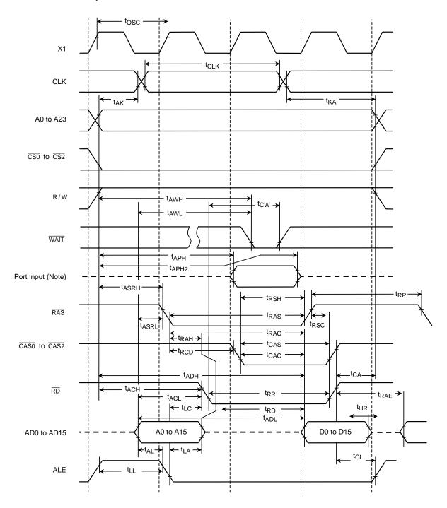
Note: Since the CPU accesses the internal area to read data from a port, the control signals of external pins such as  $\overline{\text{RD}}$  and  $\overline{\text{CS}}$  are not enabled. Therefore, the above waveform diagram should be regarded as depicting internal operation. Please also note that the timing and AC characteristics of port input/output shown above are typical representation. For details, contact your local Toshiba sales representative.
