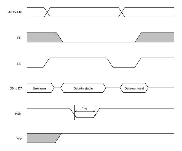
Note 1: The power supply of  $V_{PP}$  (12.75 V) must be turned on at the same time or the later time for a power supply of  $V_{CC}$  and must be turned off at the same time or early time for a power supply of  $V_{CC}$ .
