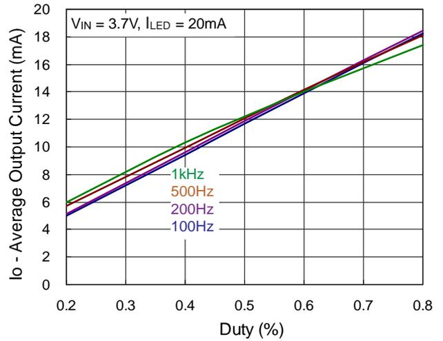
Dimming Operation for 3LEDs
