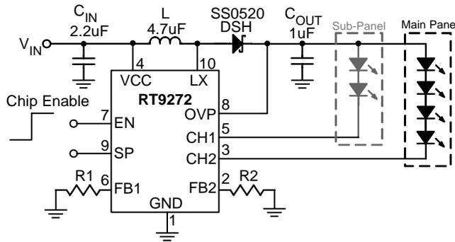
Figure 1. 2LEDs for Sub panel and 4LEDs for Main panel
