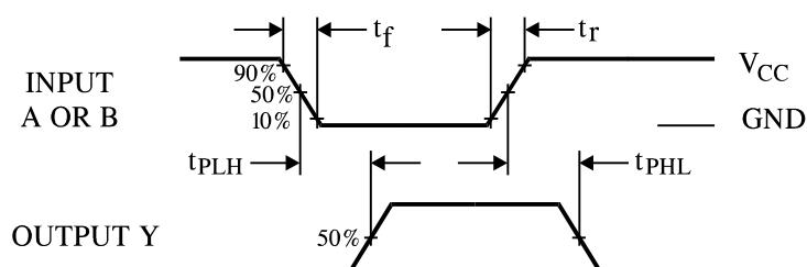
**Figure 1. Switching Waveforms**
