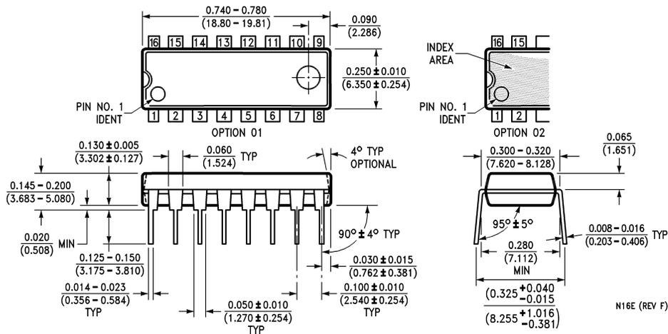
**16-Lead Molded Dual-In-Line Package (N)**
