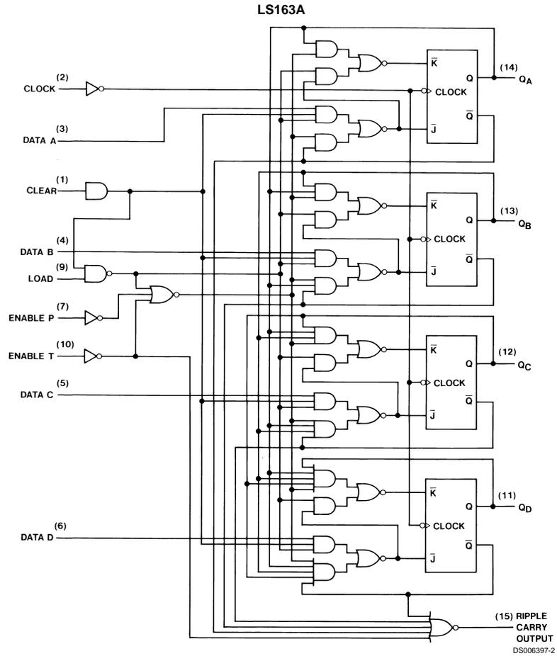
The LS161A is similar, however, the clear buffer is connected directly to the flip flops.
