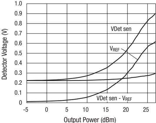
**Built-In Detector Responses at  $V_{CCDet} = 2.5 V$**
