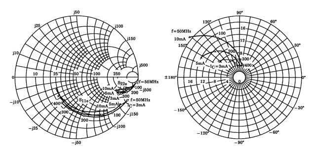
$\begin{array}{c} S_{12e} \\ V_{CE} = 10V \\ Ta = 25^{\circ}C \end{array}$
