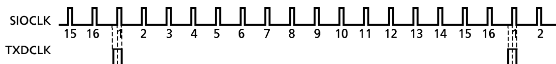
Figure 3.8.12 Generation of Transmission Clock
