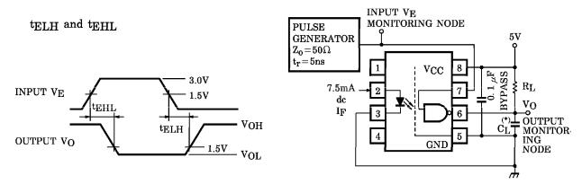
(\*) CL is approximately 15pF which includes probe and stray wiring capacitance.
