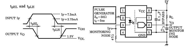
(\*) CL is approximately 15pF which includes probe and stray wiring capacitance.
