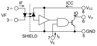
A 0.1µF bypass capacitor must be connected Between pins 8 and 5.(See Note 1)
