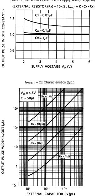
Output Pulse Width Constant K – Supply Voltage (typical)
