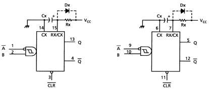
Note 1: Cx, Rx, Dx are external capacitor, resistor, and diode, respectively.
