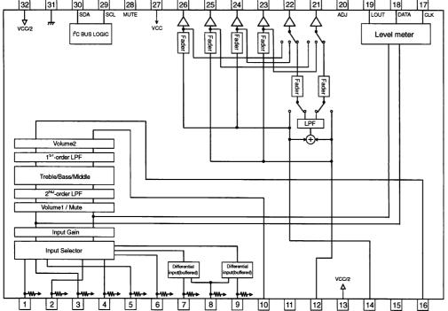
Terminal Terminal No. name 1 Α1 2 A2 B1 3 4 B2 C1 5 6 C2 7 DP1 8 DN 9 DP2 10 VOUT2 11 NC 12 FIN2 13 **FBIAS** 14 FIN1 15 NC 16 VOUT1 17 CLK 18 DATA 19 LOUT 20 ADJ OUTS2 21 22 OUTS1 23 OUTR2 24 OUTR1 25 OUTF2 26 OUTF1 27 VCC 28 MUTE 29 SCL 30 SDA 31 **GND**
