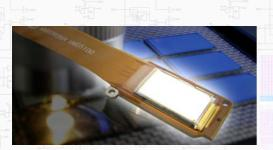
The Varitronix VMD5100 is an active matrix LCOS microdisplay with 1280 x 720 spatial resolution and 0.7" in diagonal. It is designed and fabricated using standard CMOS VLSI technology. It supports 5V liquid crystal driving and thus enhances flexibility in using different liquid crystal optical modes. VMD5100, which is integrated with proprietary driving scheme and new gamma correction algorithm, enriches image quality and enhances color depth.
