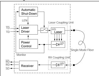
The receiver component converts the optical serial data into PECL compatible electrical data (RD and RDnot). The Signal Detect (SD, active high) shows whether optical data is present<sup>(1)</sup>.
