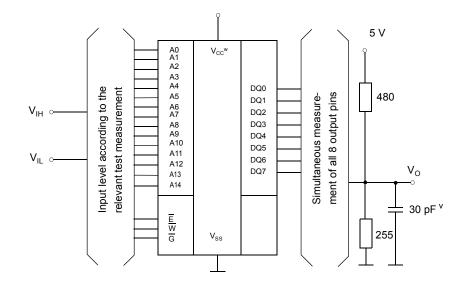
v: In measurement of  $t_{dis}$ -times and  $t_{en}$ -times the capacitance is 5 pF.
