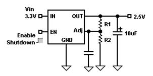
A capacitor from Adj to Ground provides greatly improved noise performance.
