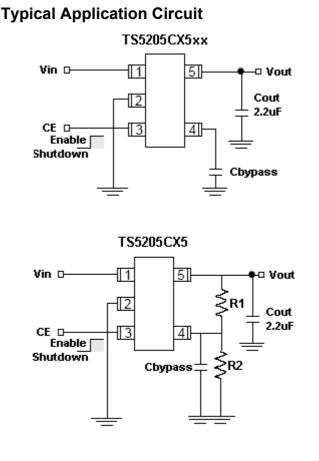
CE (pin 3) may be connected directly to Vin (pin 1) Low noise operation: Cbypass=470pF, Cout>2.2uF Basic operation: Cbypass=not used, Cout>1uF
