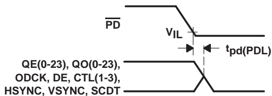
Figure 7. Delay From \overline{PD} Low to Hi-Z Outputs
