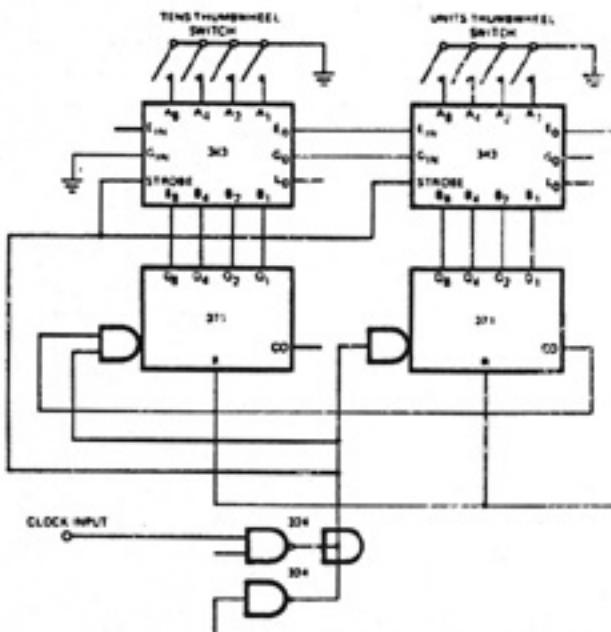
In this example, the counter modulus is any number up to 99 set with two thumbwheel switches. When the counters reach this number, the second comparator's  $E_{out}$  resets the counters. The 343 strobe inputs are tied to the system clock to prevent the possibility of false comparisons being made when the counters are changing state.
