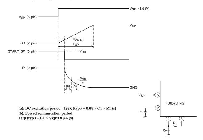
The rotor is aligned to a known position in DC excitation mode for period (a), during which the IP pin voltage decreases to half  $V_{DD}$  level. The time constant for the period is determined by  $C_2$  and  $R_1$ . After that, switching occurs to forced commutation mode represented by (b). The duty cycles for DC excitation
