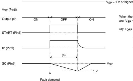
When the SC pin capacitor =  $0.47 \mu F$ and  $V_{SP} = 4 V$
