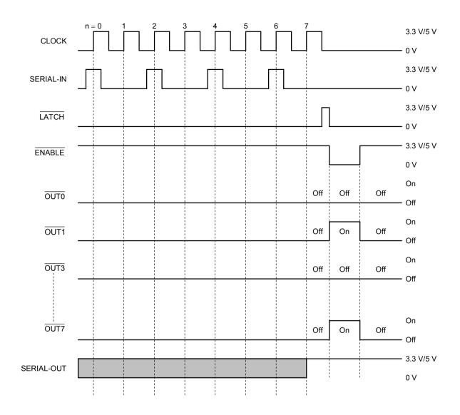
Warning: Latch circuit is leveled-latch circuit. Be careful because it is not triggered-latch circuit.
