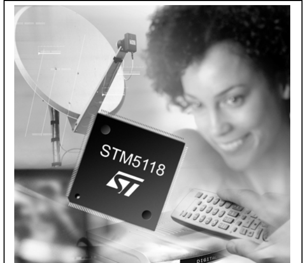
Figure 1. Package (24 x 24 mm LQFP216)
