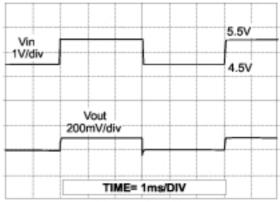
NOTE:  $V_{CC}$  = 4.5 to 5.5V,  $I_{OUT}$  = 30 mA
