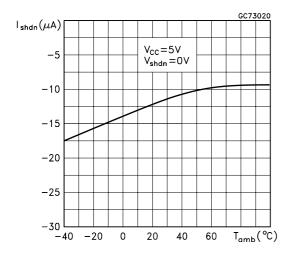
Figure 5 : SHDN Pin Current vs Temperature
