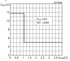
Figure 8 : Output Voltage vs Shutdown Input Voltage
