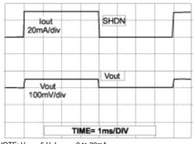
NOTE:  $V_{CC} = 5 \text{ V}$ ,  $I_{OUT} = 0 \text{ to } 30\text{mA}$
