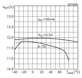
Figure 2 : Output Voltage vs Temperature
