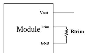
Equation for calculating the trim voltage (in V) given the desired adjusted voltage (Vadj) is shown below. The Trim Up voltage should be connected between the Trim pin and Ground.
