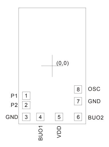
Note: The substrate MUST be connected to Vss in PCB layout.
