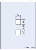
The recommended thickness of the screen mask for soldering is between 100 and  $200\,\mu m$ . The hole size of the screen mask should be same as the recommended land pattern or smaller.
