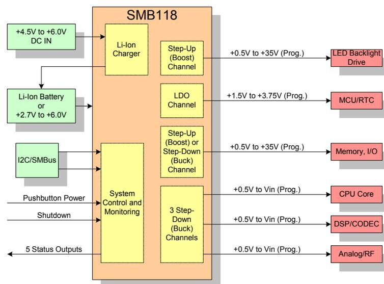
**Figure 1 – Applications block diagram featuring the SMB118 six-channel, programmable DC/DC converter. This integrated power supply and battery manager provides precision regulation, monitoring, cascade sequencing, output margining and battery charging.**
