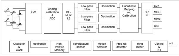
Figure 1 SCA3000-D01 Block Diagram
