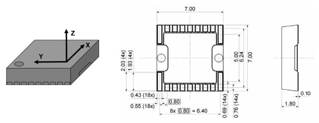
**Figure 2** Sensing directions and package dimensions in mm with ±50 µm tolerance.
