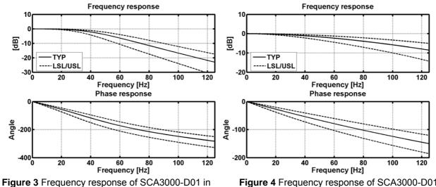
Figure 3 Frequency response of SCA3000-D01 i measurement mode
