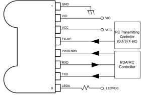
(2) RC transmitting mode at IDA receiver active condition
